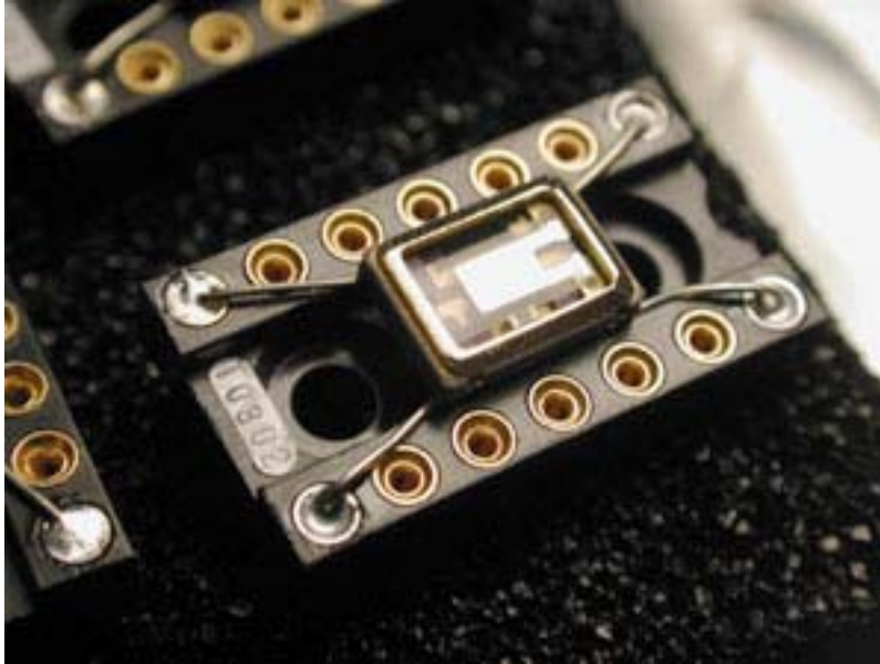
Photo 3. Cardinal CPPC7L-BP-1.2TS 5x7mm, programmable oscillator programmed to 1.2MHz and 3.3V. The quartz crystal, which is approximately 75 microns thick, is on top of the CMOS die (the translucent rectangle with aluminized electrodes).
