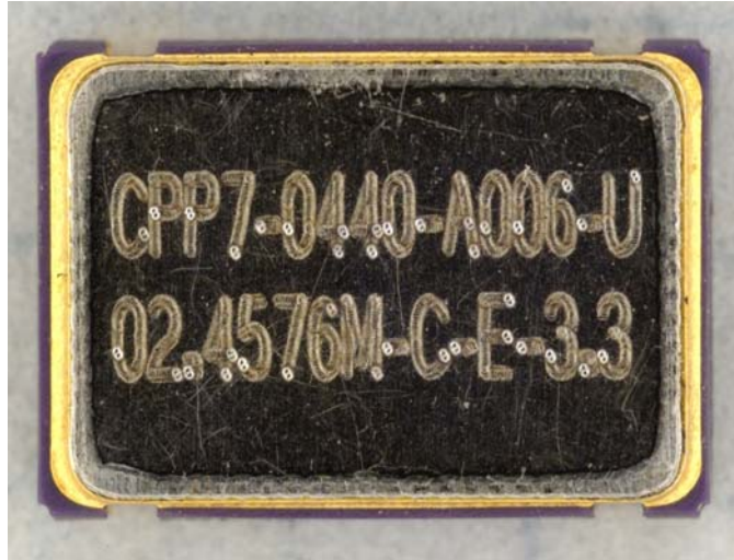
Figure 1: Example of marking on an actual FIPO, 5x7 ceramic package programmed in the 40 th week the year 2004, serial number is A006, up-screened. The programmed values were 2.4576 Mhz for the frequency, CMOS output, device is enabled at 3.3V supply.
