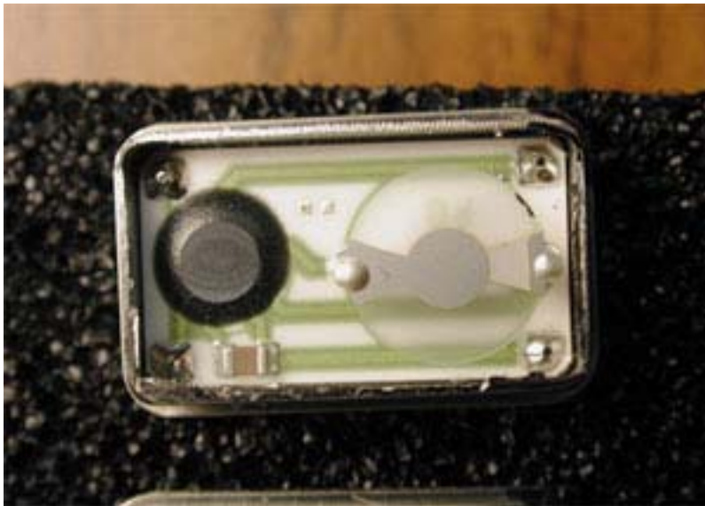
Photo 4. Cardinal CPPC1 full-size can package with the top removed shows the crystal (translucent circle on the right) and the epoxy "glop" (black circle on the left). The peak of the epoxy "glop" was milled down to reduce the amount of material that the ions had to pass through prior to hitting the CMOS die.
