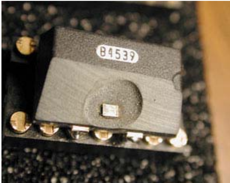
Photo 2. Cardinal CPPC8 plastic SMD, programmable oscillator programmed to 1.0MHz and 3.3V. Part of the plastic packaging was etched away so that the CMOS die is fully exposed.
