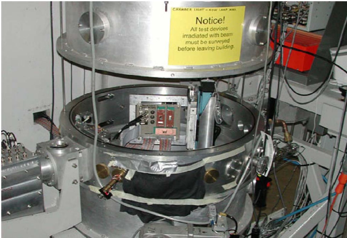
Photo 1. Cardinal Oscillator test board (with three DUTs installed) mounted in the Texas A&M University Cyclotron Institute Radiation Effects Test Facility vacuum chamber.
