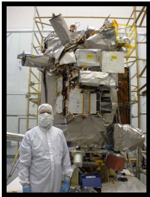
+Y Panel with Optical Bench
