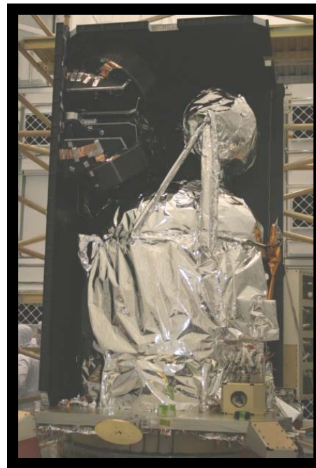
Propulsion Module with -Z ; -Y; +X Panels
