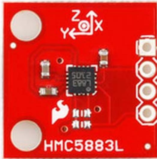
Figure 11: Magnetometer
