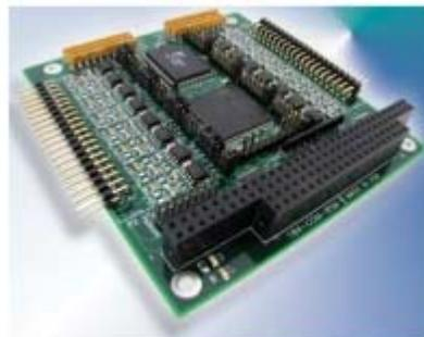
Figure 40: Accesio 104-COM-8SM Communication Board
