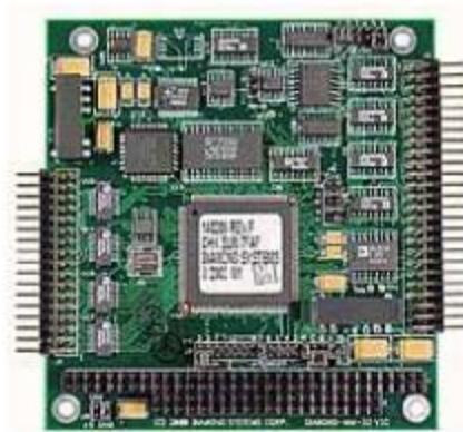
Figure 41: Diamond-MM-32-AT I/O Transceiver Board
