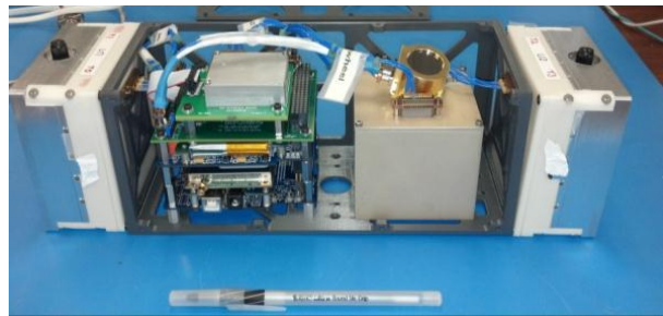
Figure 7 - Cubesat Assembly with Hardware Before Final Integration
