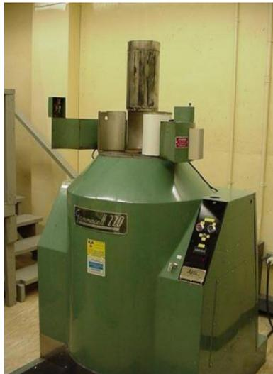
**Figure 2-11: Gammacell 220 Radiation Chamber**
