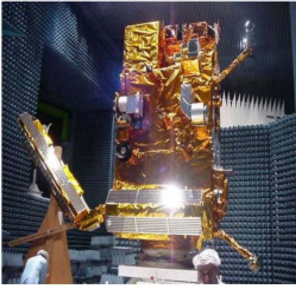
Figure 4. EMC testing of the METOP EQM spacecraft.
