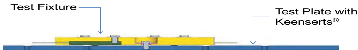
Figure 1. Bolt Preload Test Fixture & Test Plate
