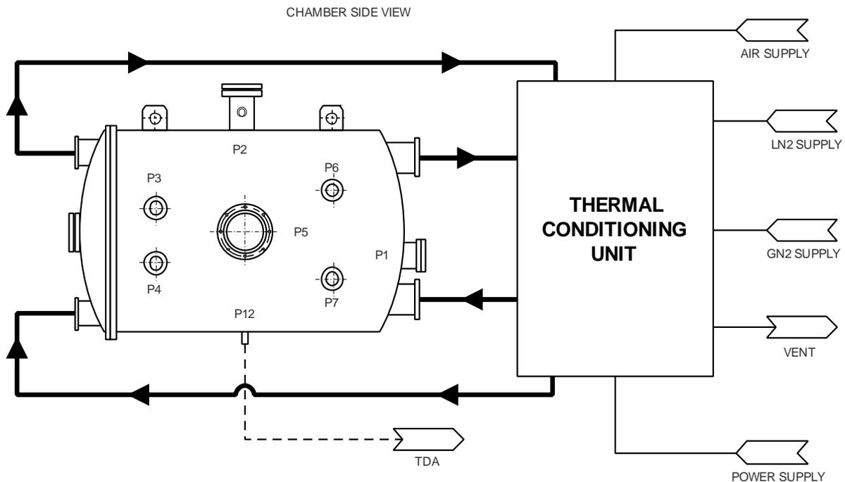
**Figure 8. Thermal System – Thermal Vacuum Chamber X**
