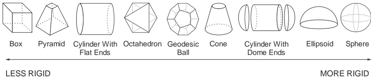
**Figure 5. Types of vacuum chamber shapes and rigidity level of the shapes. Adapted <sup>8</sup>**
