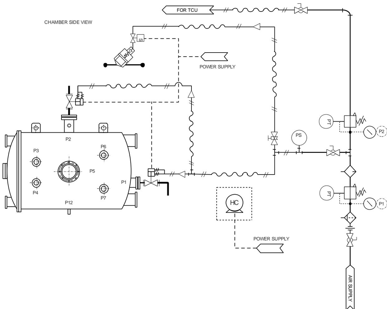
**Figure 13. Compressed Air distribution – Thermal Vacuum Chamber X**
