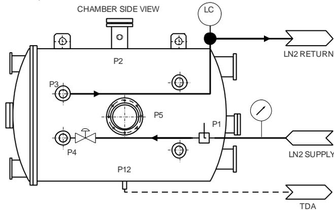
**Figure 11. Decontamination System - Thermal Vacuum Chamber X**
