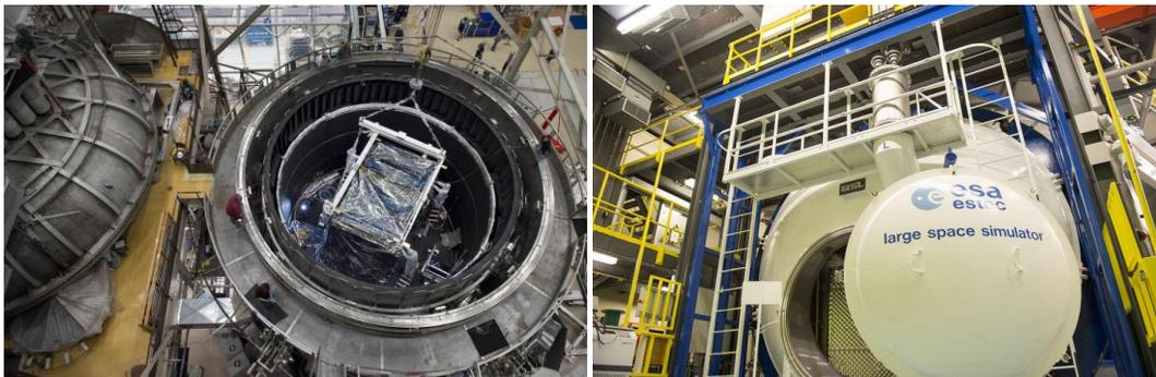
**Figure 2. (Left) Space Environment Simulator (SES) NASA Goddard Space Flight Center and (Right) Large Space Simulator (LSS) ESTEC Test Centre, ESA.**
