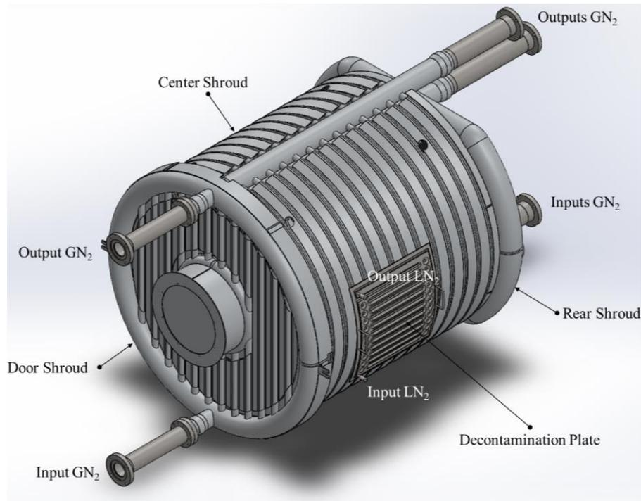
**Figure 10. Thermal System - Thermal Shrouds – Door, Center and Rear Shroud.**
