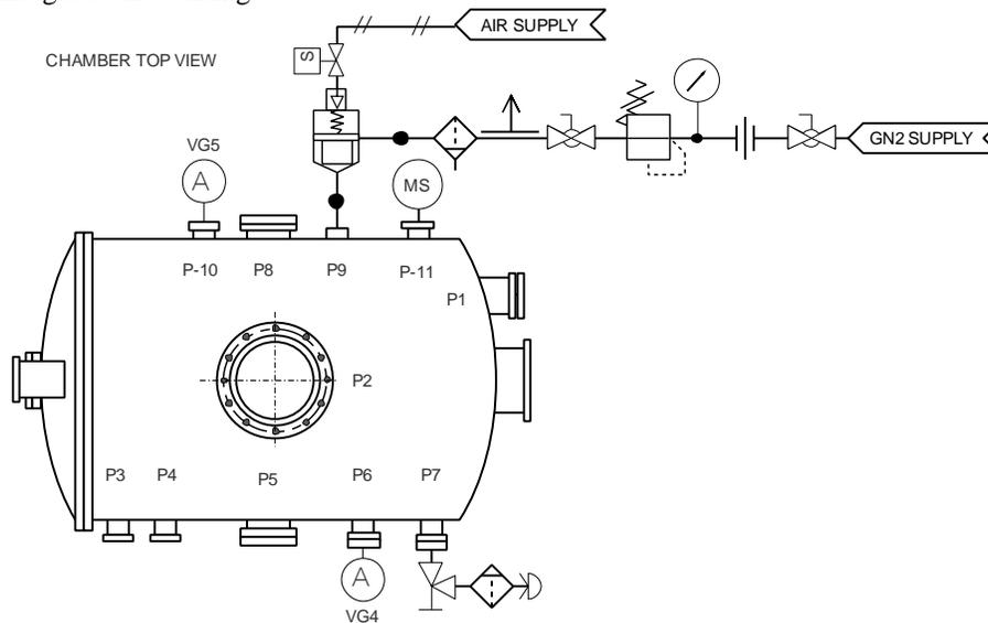
**Figure 12. Venting System – Thermal Vacuum Chamber X**
