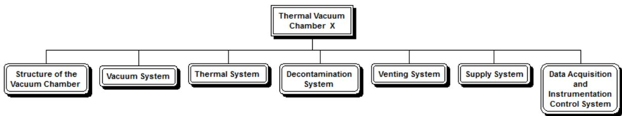
**Figure 4. Systems that integrate the Thermal Vacuum Chamber X.**
