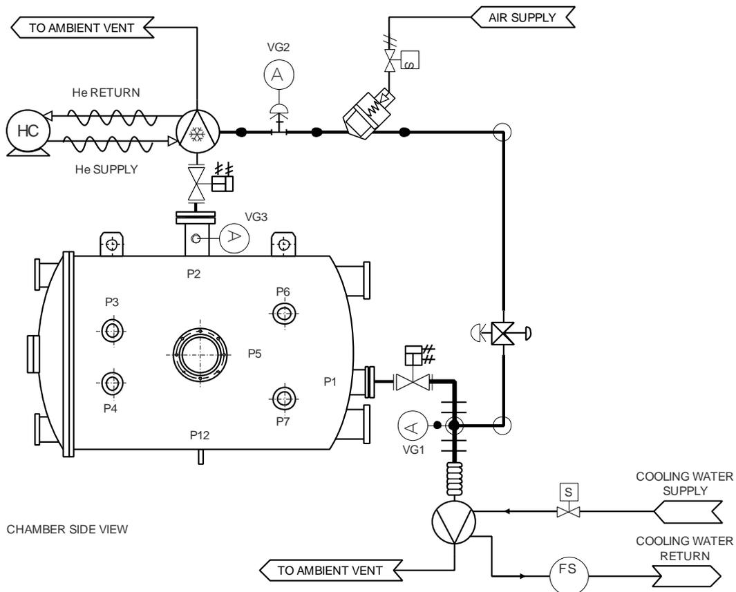
**Figure 7. Vacuum System - Thermal Vacuum Chamber X**
