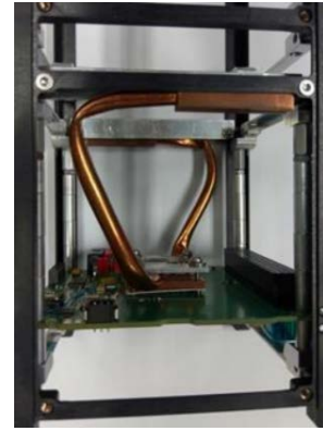
Figure 2. ISIS' CubeSat heat pipe. An example of a High-Power SmallSat thermal control technology.
