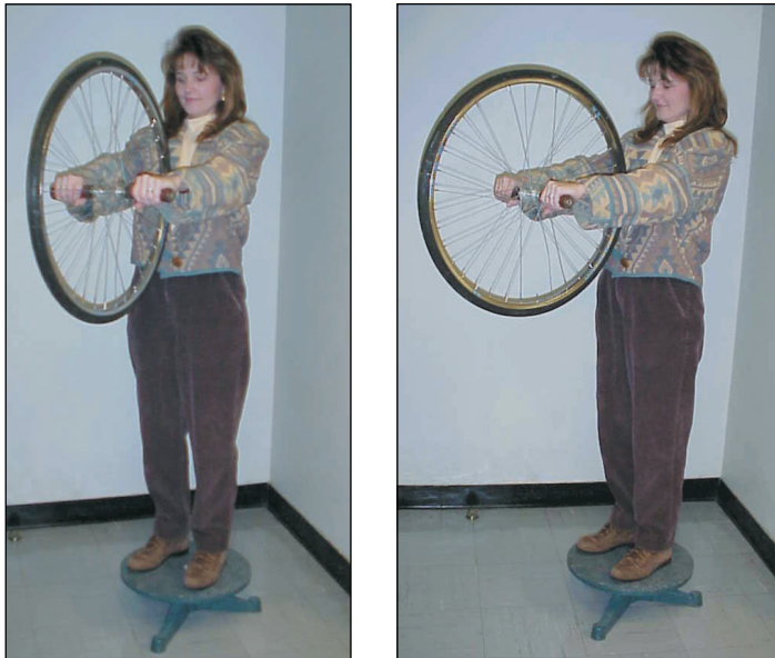
Figure 4.3.1-31. Bicycle Wheels in Space? You can do a simple experiment to see one way spacecraft control their attitude. By standing on a turntable and holding a spinning bicycle wheel, as shown in the left-hand photograph, you can change direction (your attitude). You'd simply apply a small torque to the wheel by slightly tilting the wheel to one side, as shown in the right-hand photograph.
