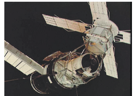
Figure 4.3.1-36. A Control Moment Gyroscope (CMG) in Space. CMGs can vary the magnitude and direction of their angular momentum, allowing for much higher slew rates and making possible efficient attitude control on very large platforms, such as the Skylab Space Station shown here. (Courtesy of NASA/Johnson Space Center)
