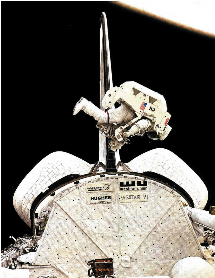
Figure 4.3.1-1. Space Vehicle Control. An astronaut flying the manned maneuvering unit (MMU) must carefully control rotation, position, and velocity to accomplish the mission (and not get lost in space!). (Courtesy of NASA/Johnson Space Center)
