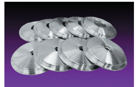
Figure 4.3.1-32. Biased Momentum Systems. We use momentum wheels in biased momentum systems. They typically rely on a single wheel with a large, fixed ("biased") momentum to provide overall stiffness. The wheel speed gradually increases to absorb disturbance torques. (Courtesy of Ball Aerospace & Technologies Corporation)
