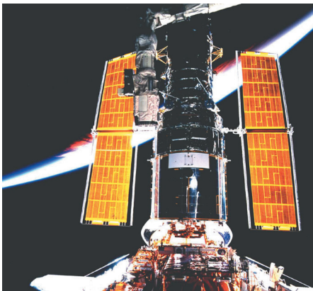
Figure 4.3.1-35. Reaction Wheels for Accurate Pointing. The Hubble Space Telescope observes many interstellar objects at such long distances that it must point very accurately. To be this accurate, it relies on very accurate reaction wheels. (Courtesy of NASA/Johnson Space Center)
