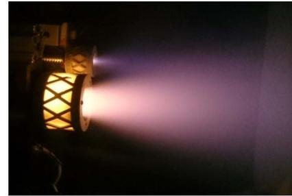
Fig. 11. Busek BIT-3 iodine thruster, from Ref. [83]
