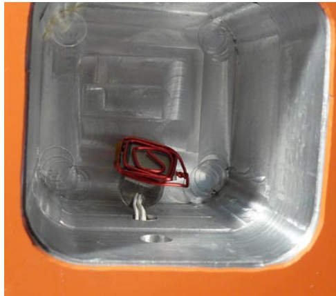
Figure 6. PEM Electrolyzer mounted inside water storage tank.
