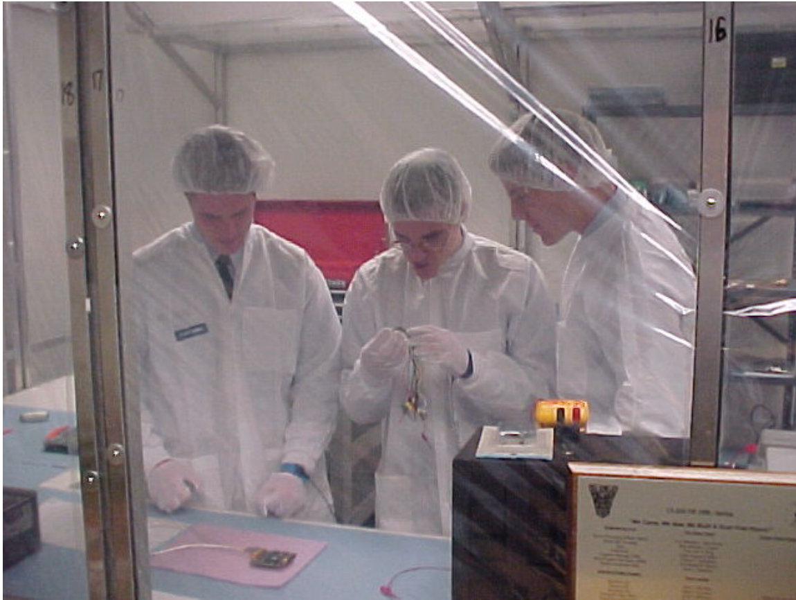
Fig. 4. Spacecraft Fabrication Activity. Cadets First Class Jim Taggart, Justin Hendricks, and Scott Karl (left to right) prepare to test the communications system modem in the small satellite clean room located in the Astronautics Laboratory at the USAF Academy.
