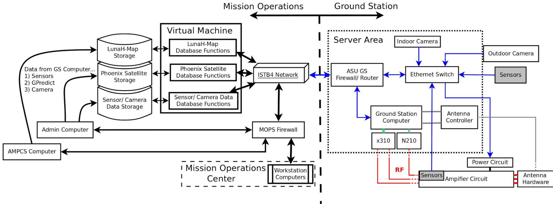
This is the ASU Ground Station's system that we plan to be working with. Phoenix data will be sorted by the network, then can be viewed by the Workstation Computers to be processed and prepared for science.
